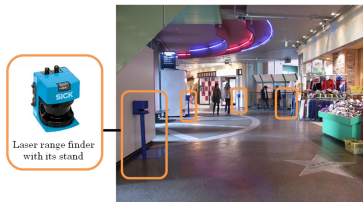
Figure 1. Example of sensor network deployed in a shopping area. Sensor poles are placed unobtrusively against walls and columns around the space to provide ubiquitous tracking.
