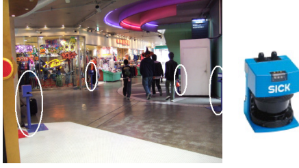
Figure 7. Experimental environment in a shopping mall. Circles indicate the installed LRF network (left). SICK LMS-200 LRF (right)
