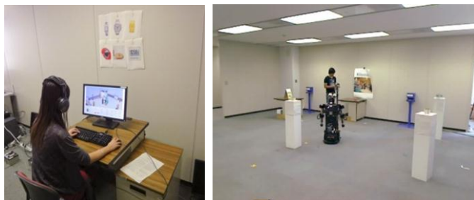
Figure 2. Photos of the experimental environment. The operator worked from a control room (left) while the robot interacted with evaluators in a separate room (right).
