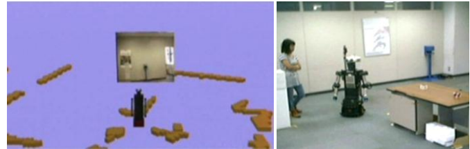
Figure 5. Interface in the No-Spatial-Visualization condition, where only laser range finder data and video from the robot's eye camera are displayed. Unless the robot is looking directly at the customer, it is difficult to identify where the customer is standing.
