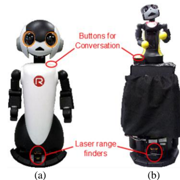
Fig. 13. Robots with buttons for conversation and laser range finders
